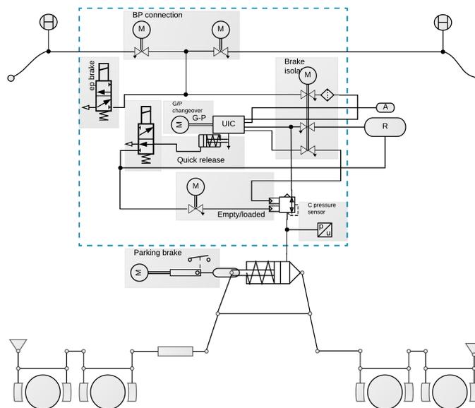
**Figure 4: Pneumatic scheme of the brake system of the Wagon 4.0**
