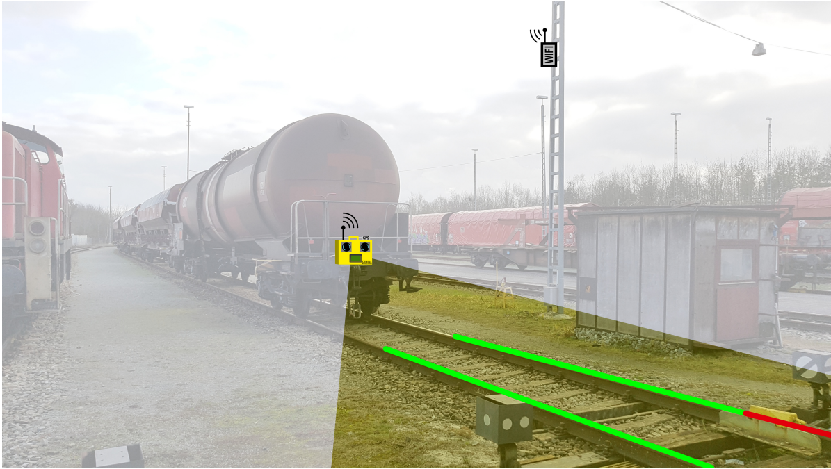
Figure 4. SAMIRA mobile temporarily mounted on the last wagon monitoring the tracks and the environment. It communicates via WIFI respectively the WMMN. Here the system detects a brake-shoe.
